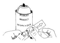
The surface preparation technique used is the same basic cleaning procedure described in Micro-Measurementss Instruction Bulletin B-129, "Surface Preparation for Strain Gage Bonding". The initial step is to thoroughly degrease with solvents such as CSM Degreaser or GC-6 Isopropyl Alcohol. CSM Degreaser is preferred whenever possible since this is a very active degreaser. The substitution of GC-6 as a degreasing agent should be considered for materials that may be sensitive to strong solvents.
