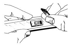
Place a silicone gum pad and backup plate (GT- 14) over the gage installation. The silicone gum should be soft (Durometer A40-60) and at least 3/32 in (2.5 mm) thick. This will allow the clamping force to be exerted evenly over the gage. The area of the silicone gum pad should be used to compute the final clamping pressure.
