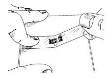
Remove the gage from its transparent envelope by grasping the edge of the gage backing with tweezers, and place bonding side down on a chemically clean glass plate or empty gage box. If a solder terminal is to be incorporated, position it on the plate adjacent to the gage as shown. A space of approximately 1/16 in (1.6 mm)
